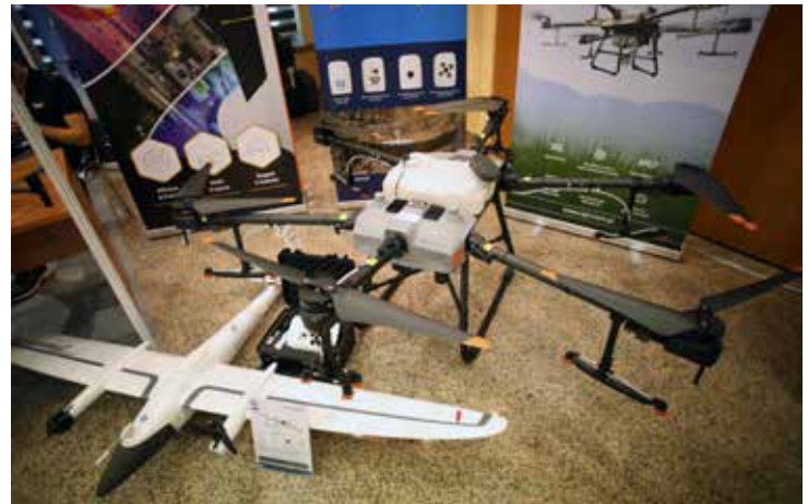
—Quantum-Systems Trinity F90+ for multi-area photogrammetry and DJI Agriculture drone used in agriculture.
