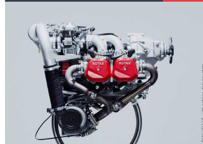
Rotax 912 ULS with options, delivery state
