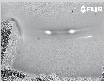
Inductive crack detection
