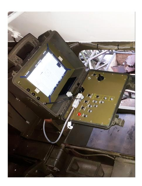
Remote control panel is designed for target selection by operator, missile launch and target tracking in manual or automatic mode with possibility of remote control up to 50 m.
