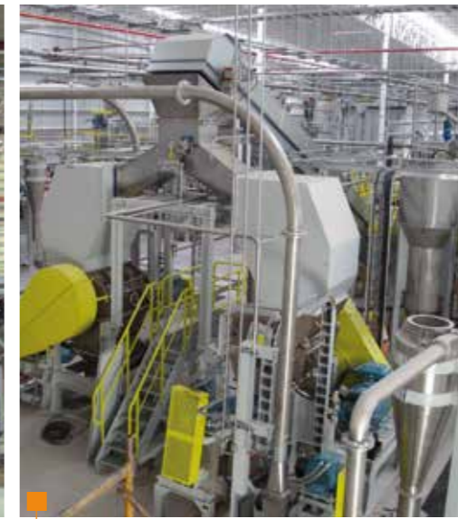
WET GRINDER: UNITS WITH HIGH FLEXIBILITY AND PERFORMANCES FOR EVERY TYPE OF PLASTICS. SPECIAL DESIGN WITH INTERCHANGEABLE WEARING PARTS.
