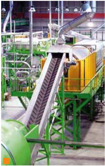
WHOLE BOTTLES PREWASHING: ELIMINATE SURFACE CONTAMINATION AND PAPER. RELEASE AND SEPARATE PLASTIC LABELS.
