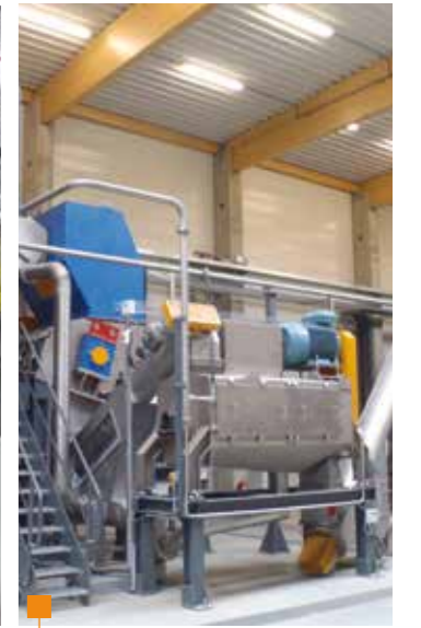
WET GRINDER: UNITS WITH HIGH FLEXIBILITY AND PERFORMANCES FOR EVERY TYPE OF PLASTICS. SPECIAL DESIGN WITH INTERCHANGEABLE WEARING PARTS.
