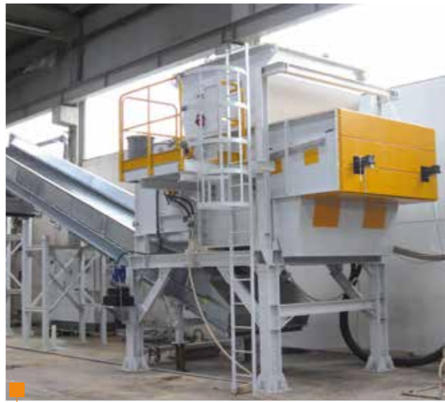
SHREDDING: FEED AT CONSTANT RATE THE WASH LINE. CONTROL SIZE AND IMPROVE PERFORMANCE IN COMBINATION WITH PREWASH.
