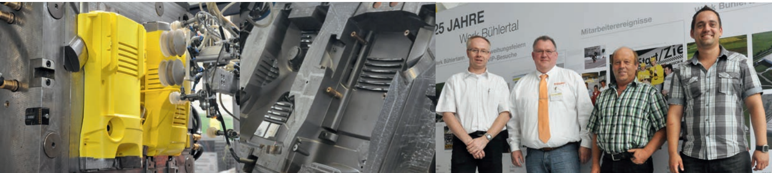
Yellow housing: 2101 parts are produced per day in the injection moulding department of Alfred Kärcher. With the help of the iQtemp cooling system, the Cycle time was reduced from 52 to 37 seconds.
