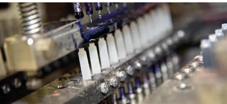
Tightly sealed: After leaving the injection moulding machine, the ink cartridges are filled.
