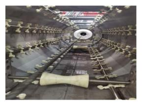
Independent servo motor control for each caterpiller with Pre-hauling winding device ,effective hauling length 2000mm
