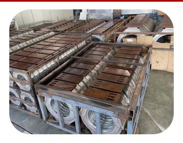
Extrusion mould is mainly composted of spiral distributor, compressing sleeve, cooling sleeve, die lip, heating and cooling control device, core temperature control system, and so on.
