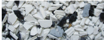
Rozdrobnione profile okienne -10 +0,5 mm PVC - 93,34%, EPDM - 6,66%
